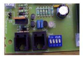
DIP switches fitted on the Ecopower board provide a selection of optional features as described above. Isolate and switch electrical power off before configuring and/or changing any DIP switch settings.
