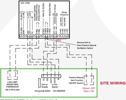
CO2 SENSOR 24v SUPPLY - Non Screened 16/0.2mm (0.5mm²) CO2 SENSOR SIGNAL - Screened 16/0/0.2mm (0.5mm²)
