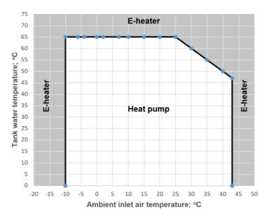
If the temperature set on the control display is more than achievable one indicated in the graph above, the E-heater will be switched ON automatically to reach it.
