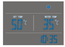
The left side of the temperature display shows the set water temperature.
